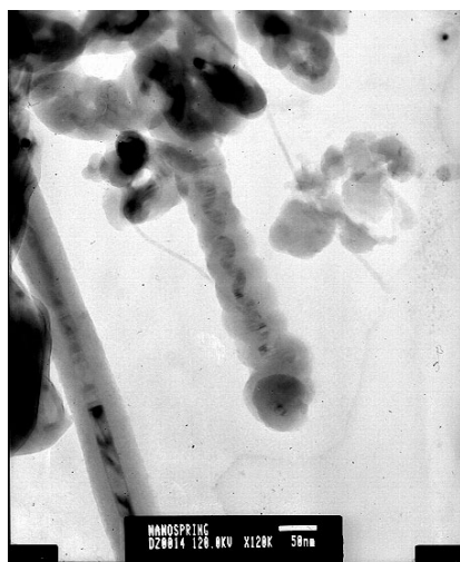
Figure 16. A TEM image of a biphase helical nanowire, which consists of a helical silicon carbide crystalline core and an amorphous silicon carbide sheath [87]. The dark region at the tip of the nanowire is the nickel silicide catalyst.
